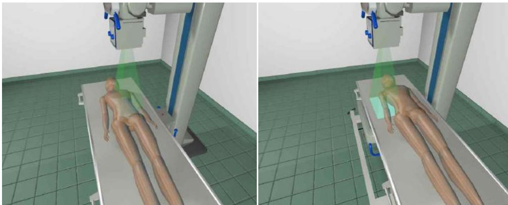
X-FRAME DR-2T: extremely wide column to detector distance makes it possible to image all anatomical districts of patients on gurneys (e.g. right and left shoulders) without the need for any risky patient movement but just by briefly translating the gurney/table over the detector.
